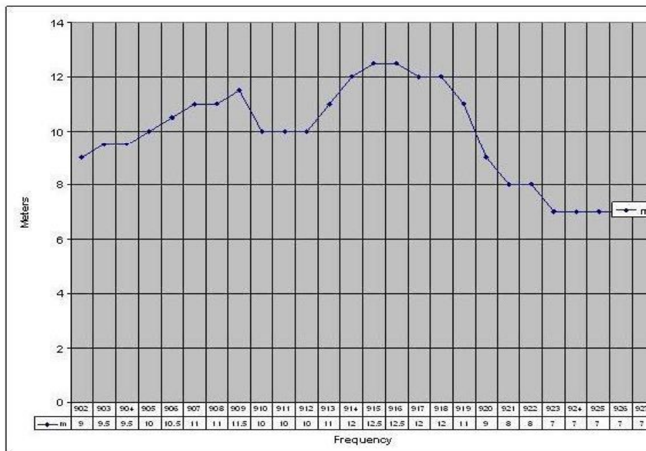
Typical read distance chart - Using a CSL101-2 handheld reader @ 90 deg from target seal
